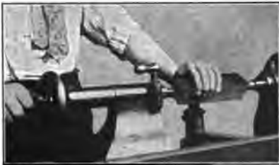
Fig. 6. Tightening the Tail-screw.
